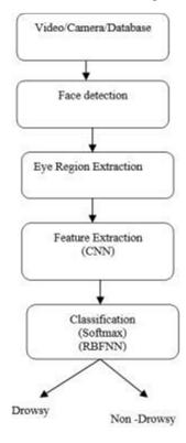
The entire face region may not be required to identify drowsiness, but merely the eyes region is sufficient. Face detection is done in the first phase using a face detection algorithm. The eye detection
