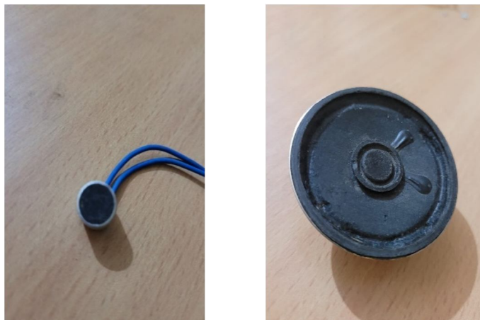
Fig. 7. Mic and Speaker
