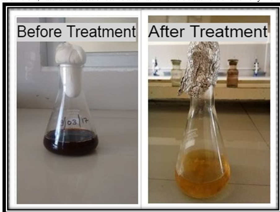
Fig. 9: Decolourization results of spent wash after PBR treatment
