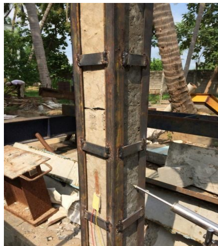
Fig 2: Crack Pattern Showing Buckling
