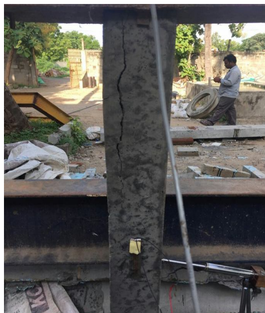
Fig.4: Steel Jacketing Setup
