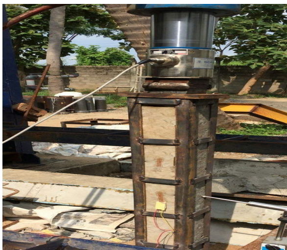
Fig.7: Model Of A Control Column With Axial Force
