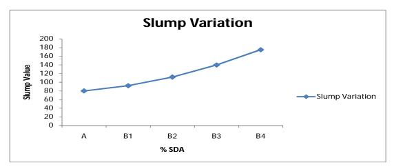
From these results it was notified that concrete becomes more workable as PEG-400 % age is increased that means less water is required to make mix more workable.
