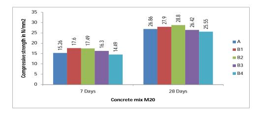
The table and graph shows the variation in compressive strength of M20 grade concrete with 0.5%, 1%, 1.5% and 2%, PEG-400 by weight of cement.
