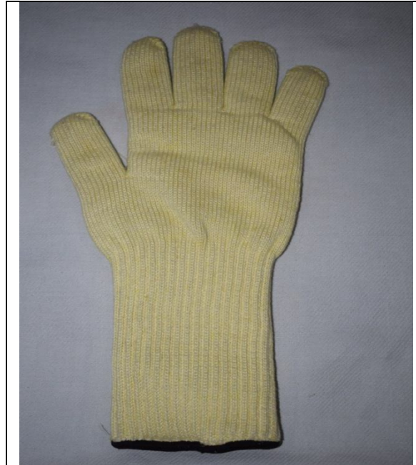
Figure 1: Para-aramid with E-glass gloves samples
