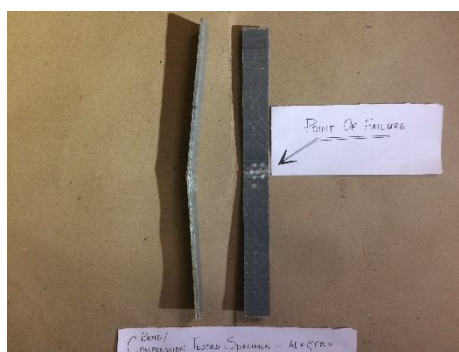
Figure.11 Sample after compression test
