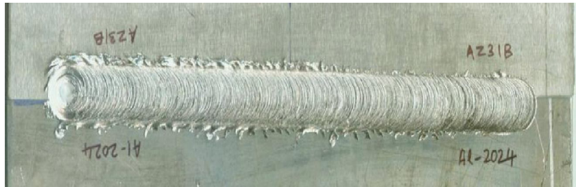
Figure 2: Surface morphology of the FSW coupon of Al alloy to Mg alloy
