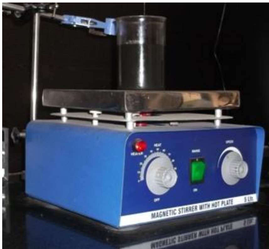
Figure 1. Experimental set-up of bio-diesel reactor with magnetic stirrer with WSO
