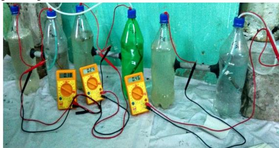
Fig. 2 Microbial Fuel Cell Setup
