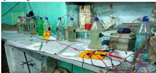
Fig. 1 Microbial Fuel Cell for the treatment of Waste water
