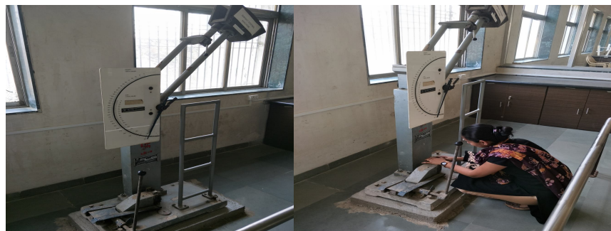
Figure 10: Charpy impact test
