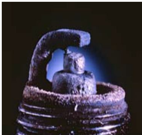
Fig. 3 Photographic view of Carbon Fouled spark plug
