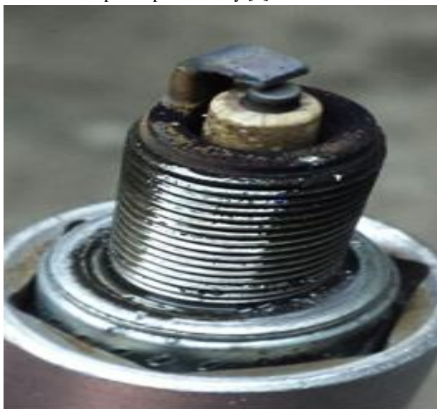
Fig. 6 Photographic view of Overheated spark plug
