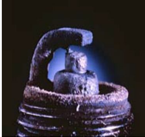
Fig. 3 Photographic view of Carbon Fouled spark plug
