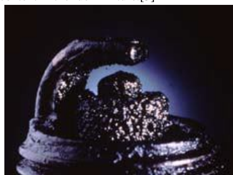
Fig. 4 Photographic view of Oil Fouled spark plug
