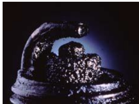
Fig. 4 Photographic view of Oil Fouled spark plug
