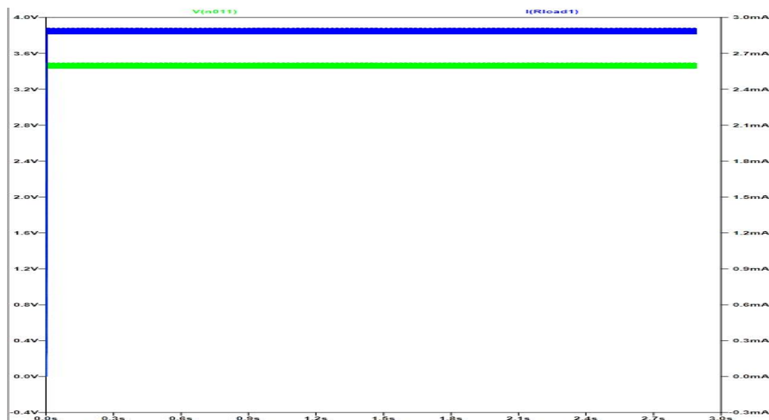
Fig.6 Piezoelectric energy harvester with continuous load current of 3ma and voltage is constant at 3.3V
