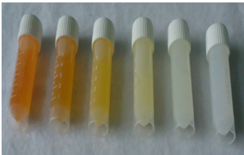
Fig. 6f: Visual change in the colour of methyl orange dye on irradiation with nano titanium oxide photocatalyst calcined at 400 °C.
