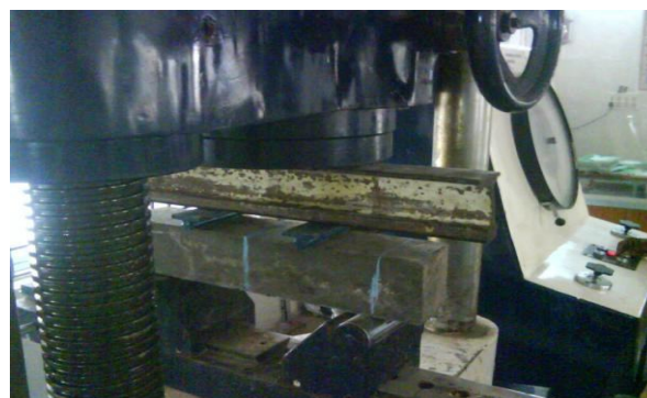
Fig 5.17 Flexural Strength with Normal Cured Specimen
