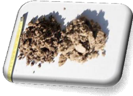
Fig 1.1 Sample of Paper Sludge of the Research
