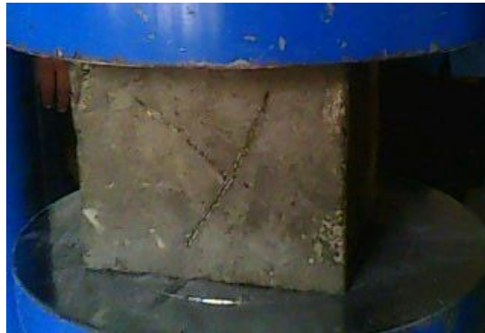
Fig. 5.12 Compressive Strength Test with Normal cured Specimen
