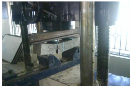
Fig 5.19 Failure Pattern of Beam in Flexural Strength Test
