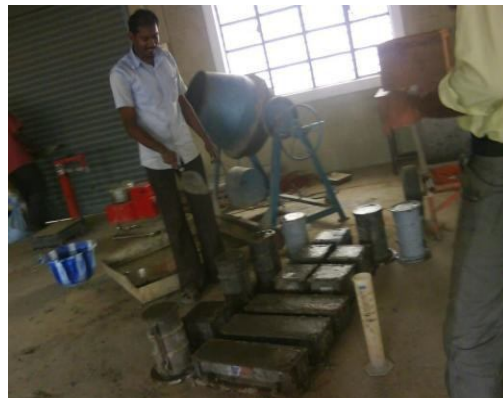
Fig 5.7 Placing of Fresh Concrete
