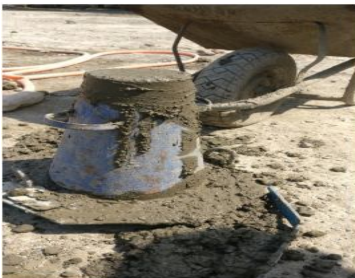
Fig.2 The slump test of concrete.
