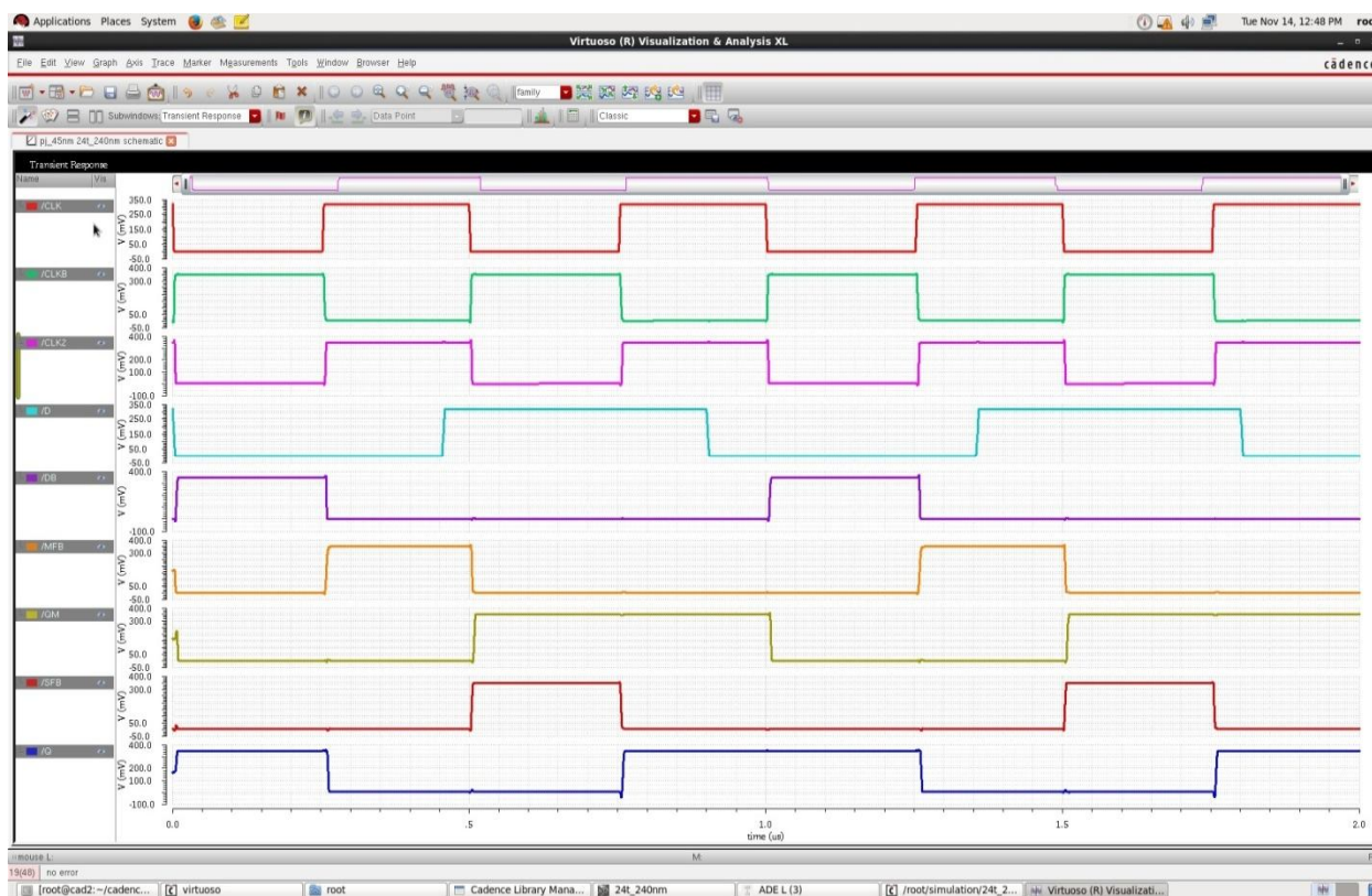
Fig.4 Timing Diagram of IVLPSFF
