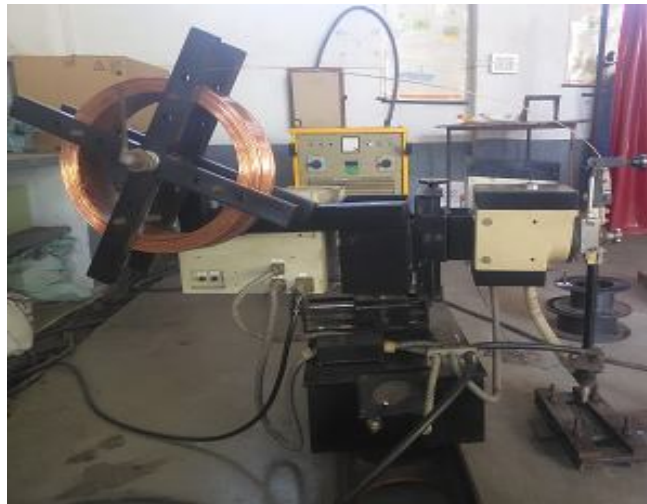
Fig. 2 Submerged Arc Welding Machine (Courtesy: Advanced welding laboratory, RIT, Rajaramnagar)
