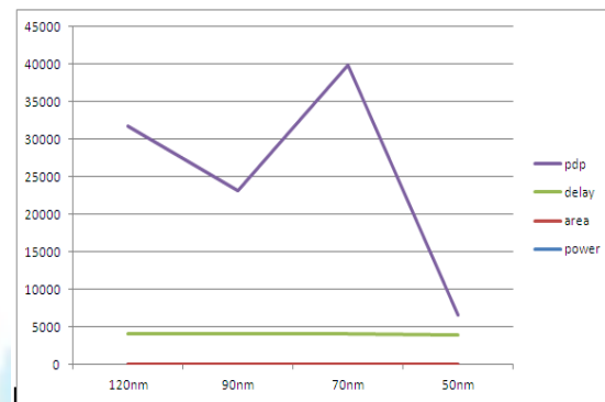
Fig17: four bit full adder dual sleep approach power & area calculations
