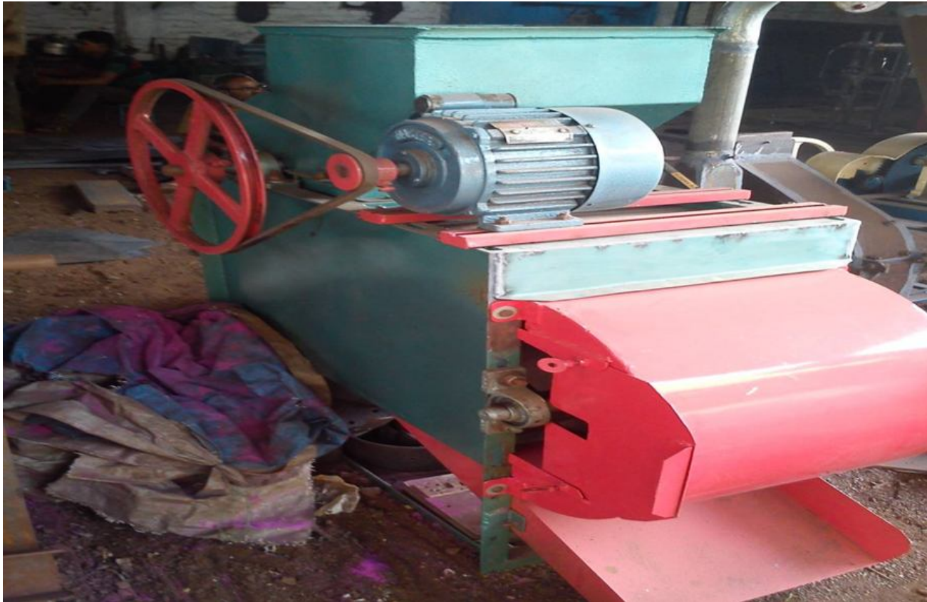
Photo 1 Final Assembly of Groundnut Decorticator
