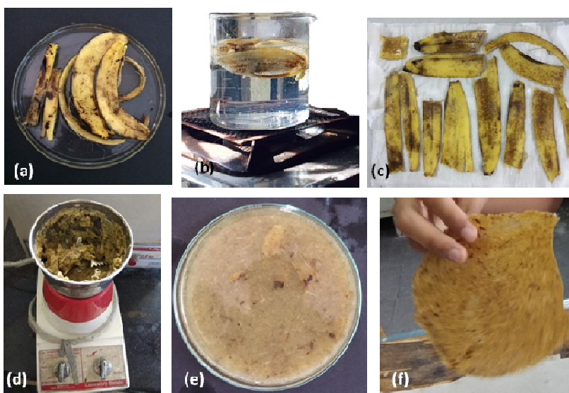
Figure 2. Processing of banana peels to produce bioplastic, (a) sodium metabisulfite treatment, (b) boiling of treated peels, (c) softened peels dried after boiling, (d) grinding into fine paste, (e) even layering onto petri dish, (f) plastic after baking in oven.
