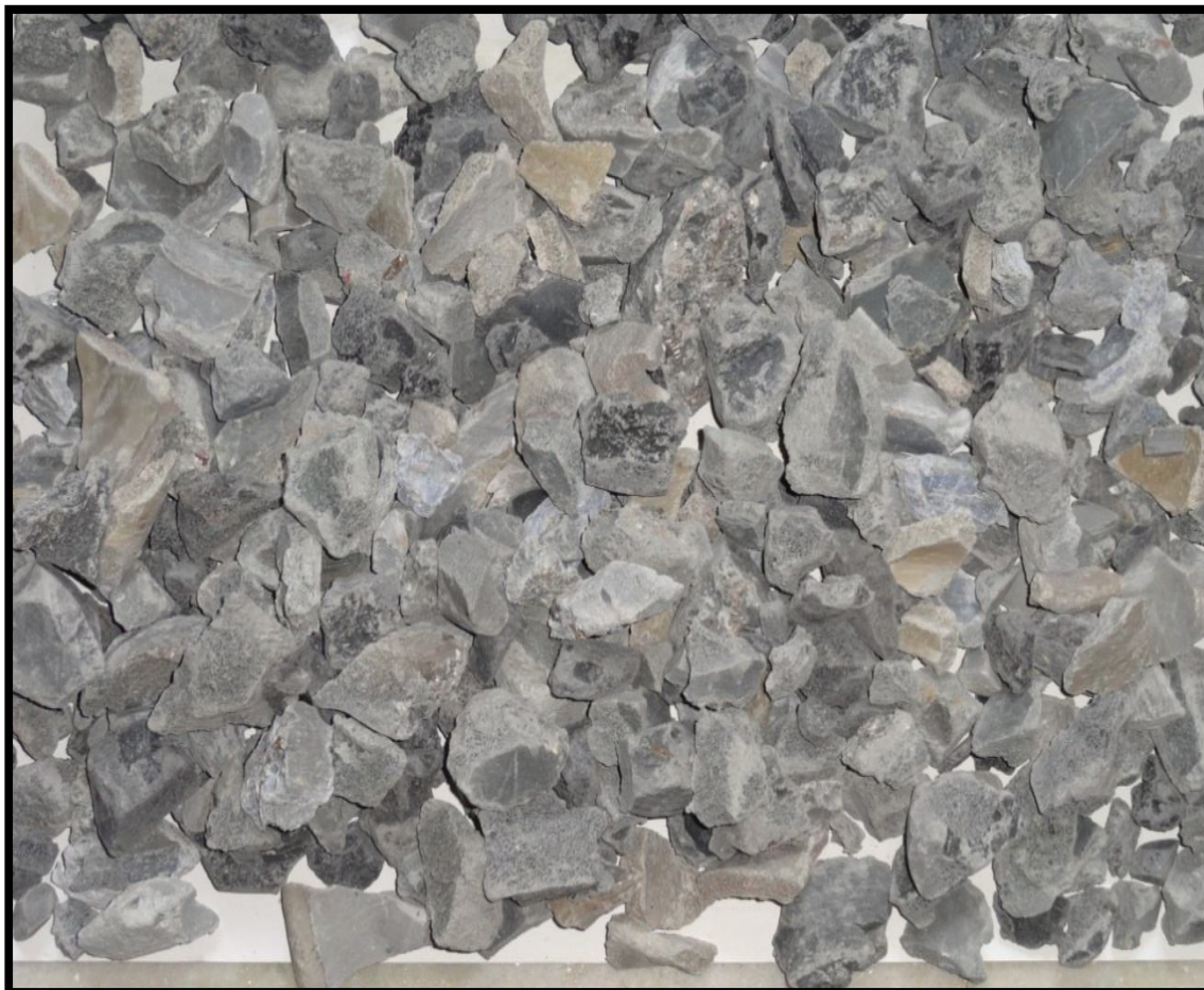
Fig.1 Waste Polymer Aggregates (WPA) derived from JaliGulla .
