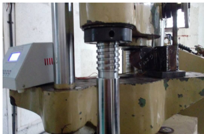
Fig. 23 Bending Loading on T-Joint
