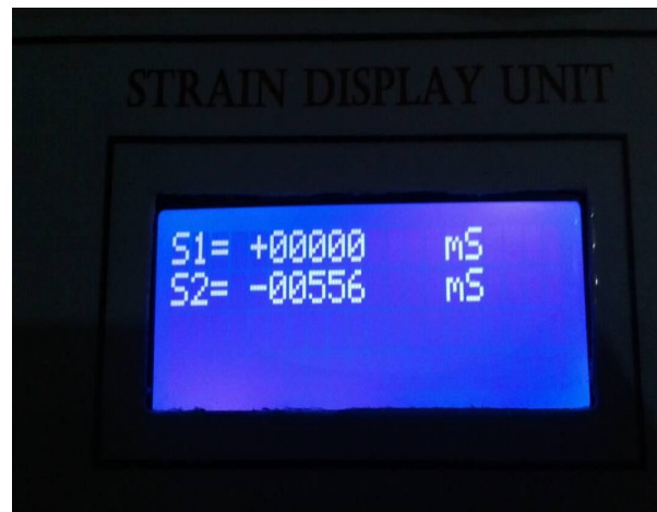
Fig. 22 Strain gage output 556 micro strains
