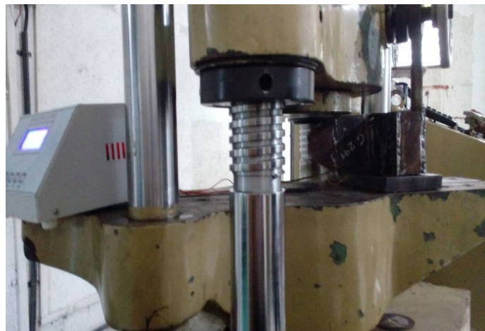
Fig. 23 Bending Loading on T-Joint
