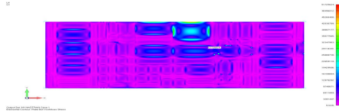
Fig: 48 Maximum Stress of 51.72 Mpa Obtained On the Bottom Plate
