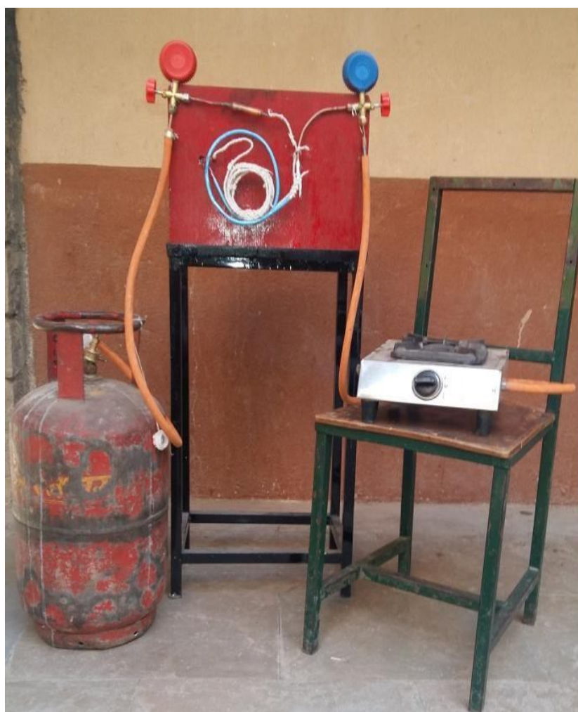
Fig.-3: Actual Setup of LPG Refrigerator
