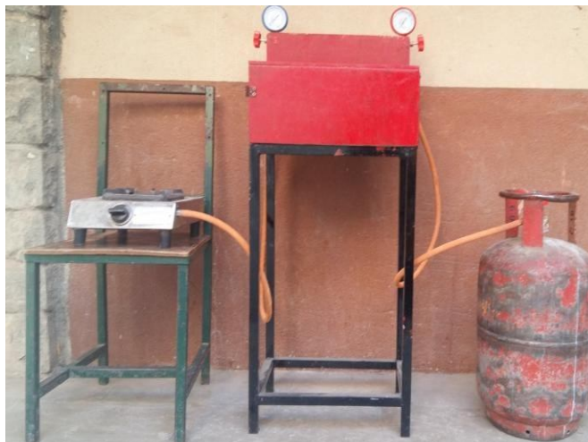
Fig.-2: Actual Setup of LPG Refrigerator
