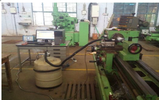
Figure 1: NAGMATI-175 lathe machine with cryocan setup
