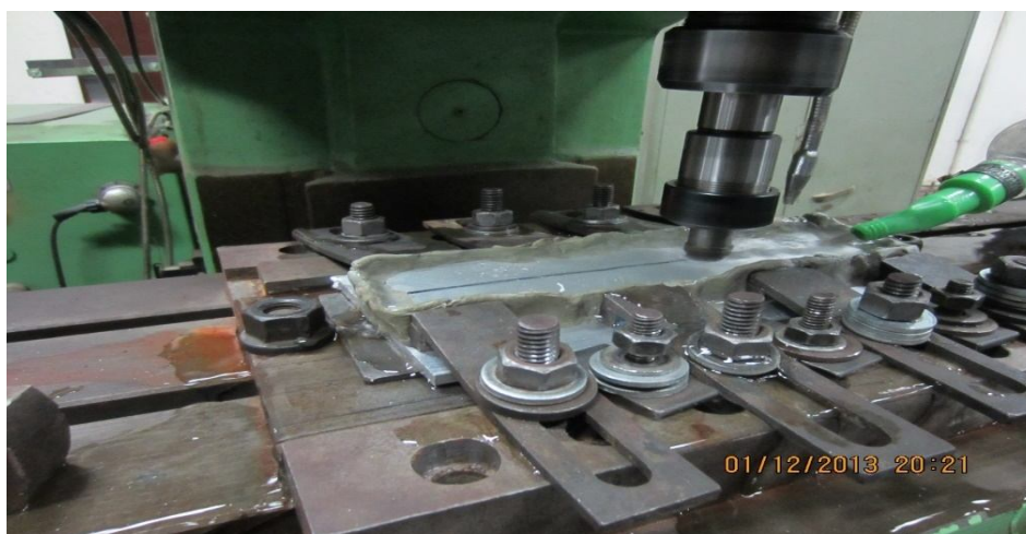
Figure 2 Setup for underwater friction stir welding
