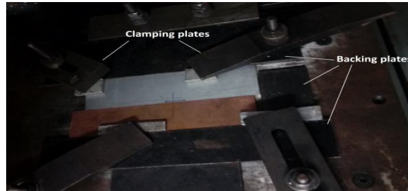
Fig. 3: Al & Cu plates clamped to the setup using backing plates.
