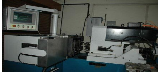
Fig. 2: Friction Stir Welding Machine at IISc
