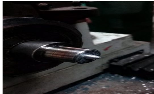
Fig. 4: Tool piece fixed to the rotor
