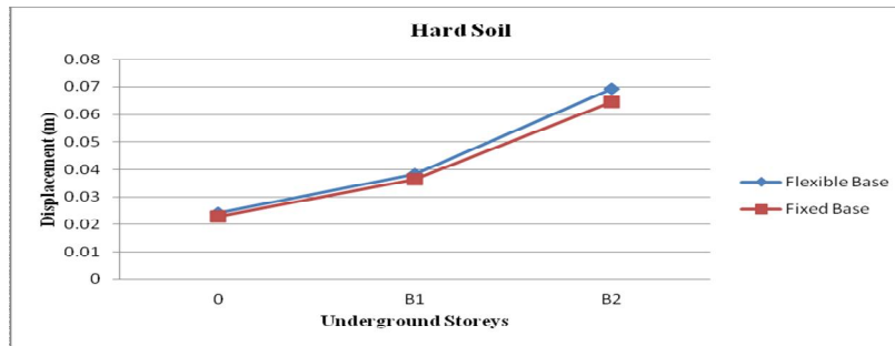
Fig. 10 Displacement values for G+5 structure with zone V for Hard Soil condition
