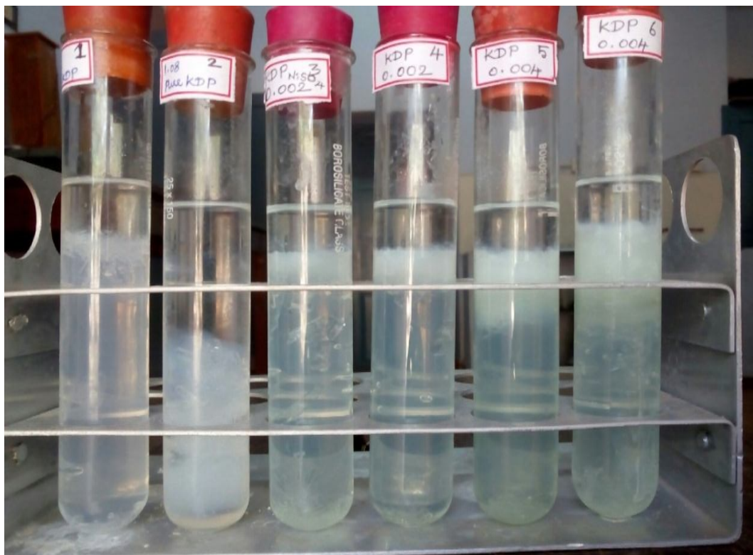
Figure.1 Growth of pure KDP doped with NiSO 4 with various concentrations
