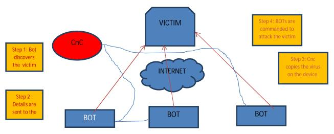
This Mirai incident illustrates how vulnerable the Internet of Things can be and demonstrates that additional security requirements are necessary to protectit from attacks and exploitation. Measures must be put in place to ensure it is securely managed, has secure communications and is monitored for future breaches.
