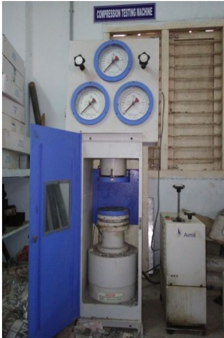
Fig. 2 Compression testing machine (CTM)
