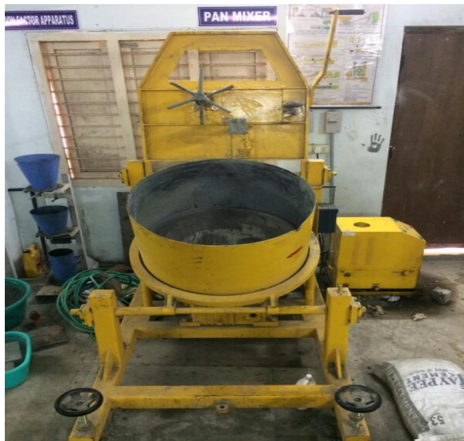
Fig. 1 Pan mixer used for mixing
