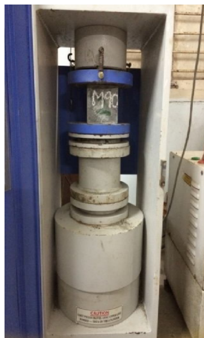
Fig. 3 Concrete cubes M 90 grade specimens in CTM
