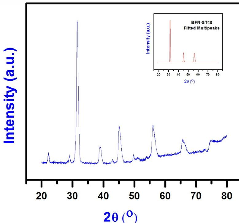
Figure .1 XRD pattern of  $0.60\text{Ba}(\text{Fe}_{0.5}\text{Nb}_{0.5})\text{O}_3-0.40\text{SrTiO}_3$  Nanoceramic system
