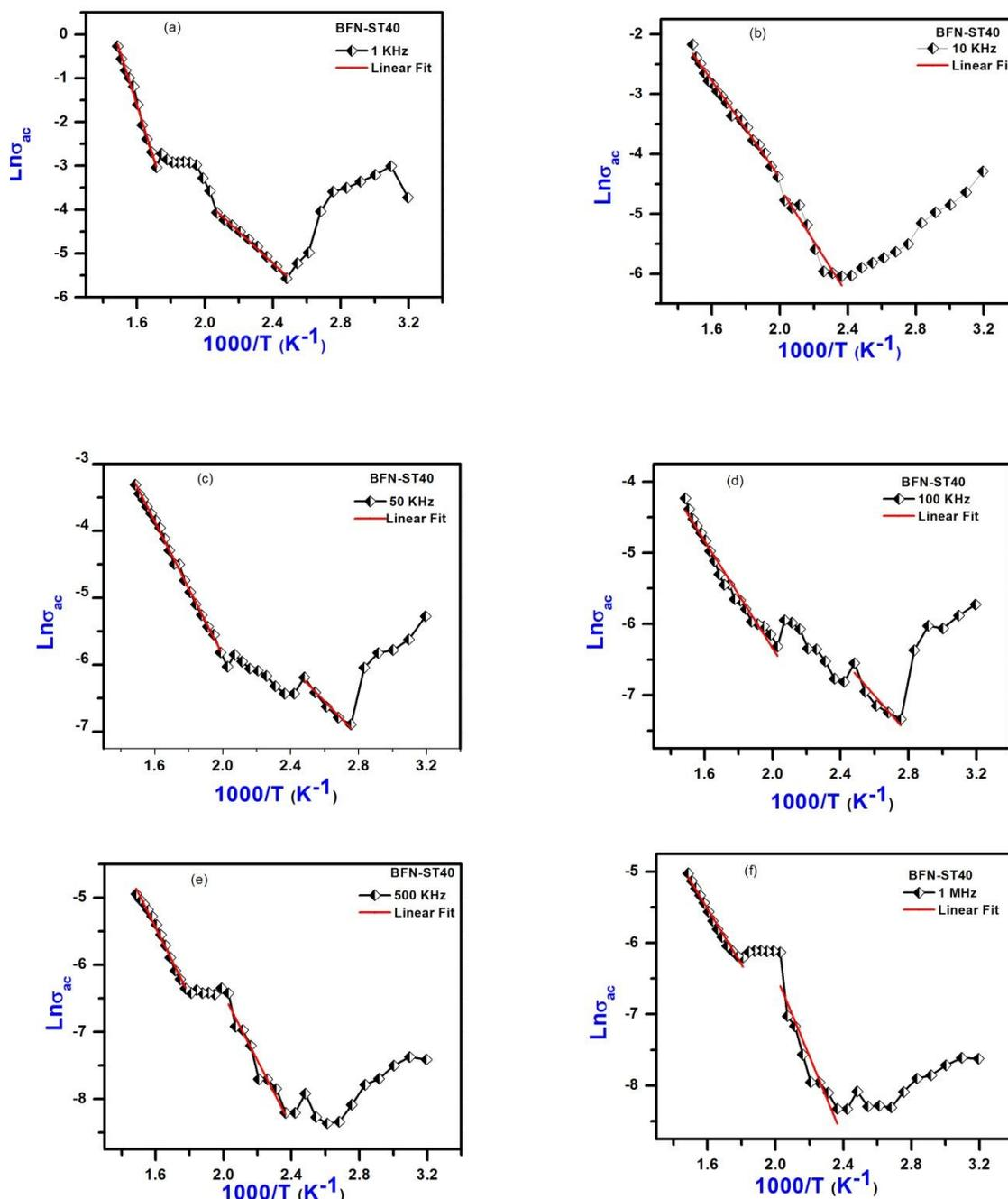
Figure 5 . AC conductivity  $\ln(\sigma_{ac})$  variation with reciprocal of temperature ( $1000/T$ ) at different frequencies for BFN-ST40 nanoceramics
