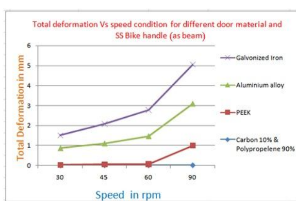
Graph 4. Total deformations Vs Speed condition for SS bike handle (as beam)
