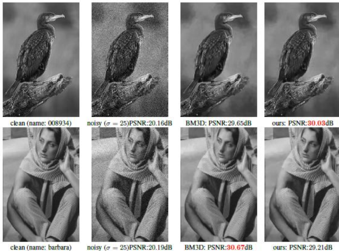
Figure 2. Our results compared to BM3D. Our method outperforms BM3D on some images (top row). On other images however, BM3D achieves much better results than our approach. The images on which BM3D is much better than our approach usually contain some kind of regular structure, such as the stripes on Barbara's pants (bottom row).
