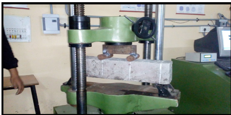
Fig. 6 Testing of beam specimen under three point loading in UTM machine
