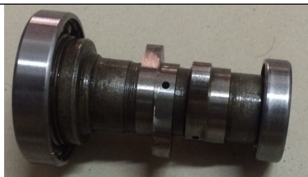
Fig.6 Actual view of the Modified cam
