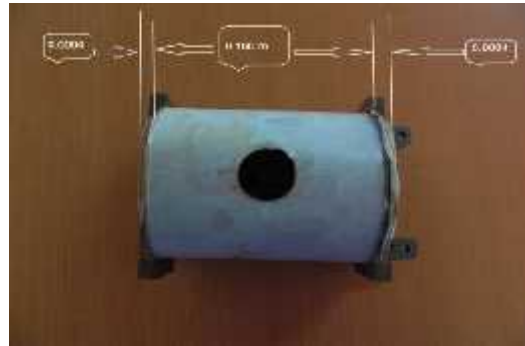
Fig 3. Deformed prototype after blast loading.
