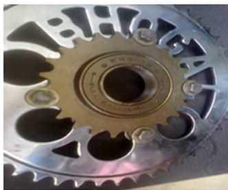
Fig.9. 48no.Tooth sprocket mounted on wheel.
