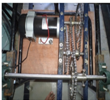
Fig.11. Complete drive train assembly
