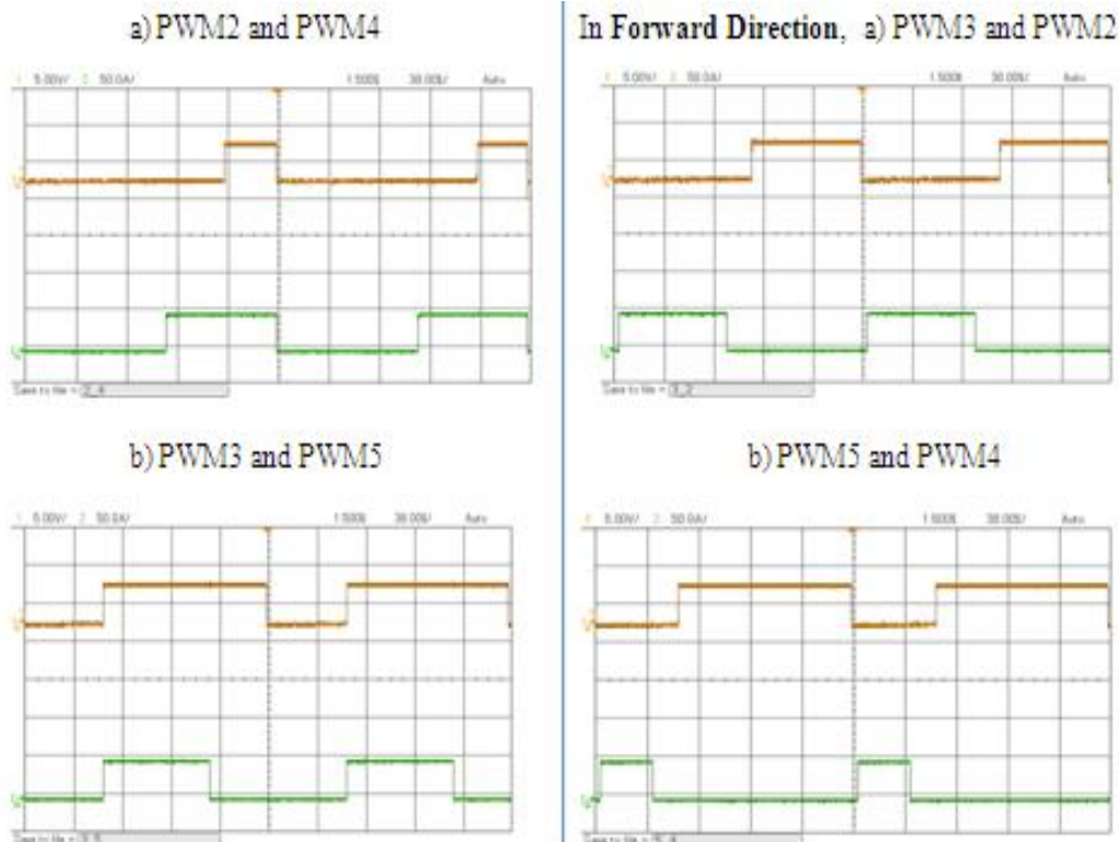
Fig. 6.7: Comparison of PWM2 and PWM3 with PWM4 and PWM5 at ADC=27
