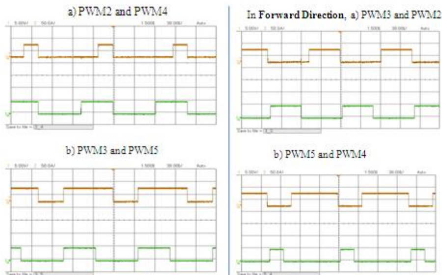
Fig. 6.6: Comparison of PWM2 and PWM3 with PWM4 and PWM5 at ADC=0
