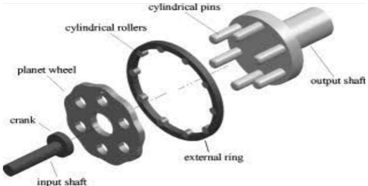
Fig:-Cycloidal speed reducer parts
