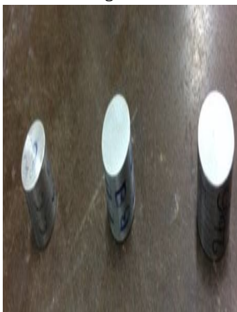
Figure 10 compacted sample of Al-6063
