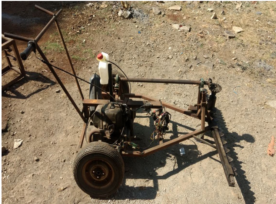
Figure1.1: our Model of the grass cutter [7].
