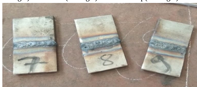
A.80Amp(50° angle) B.90A(60° angle) C.100A(70° angle)
