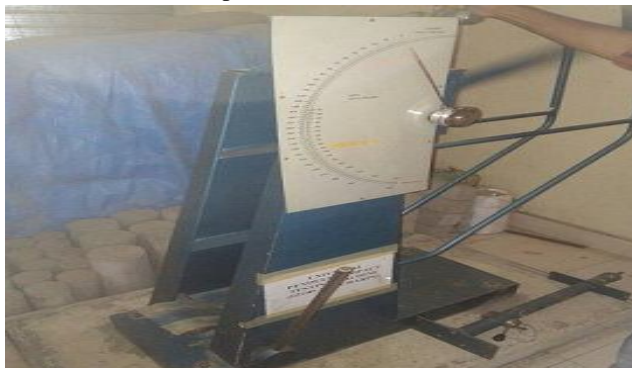
Fig. 6 Impact testing machine
