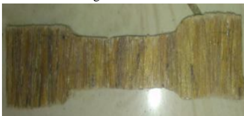
Fig 3: Test laminate of kenaf fiber
