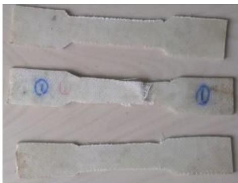
Fig: 8 E-glass specimen
