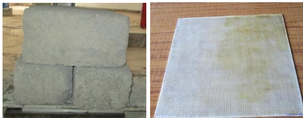
Fig 2: Weight on the mould cavity, E-Glass laminate
