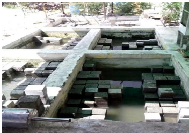
Figure 2- Casting of cubes and curing tank
