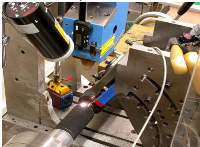
Fig.6. Laser Assisted Machining Setup
