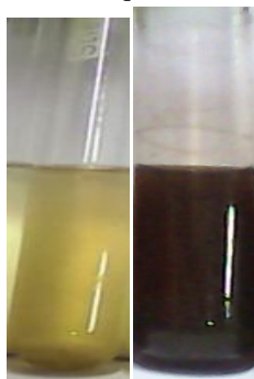
Plate 1: Digital photograph showing in the colour change of AgNO 3 on addition of aqueous extract of seaweeds.
